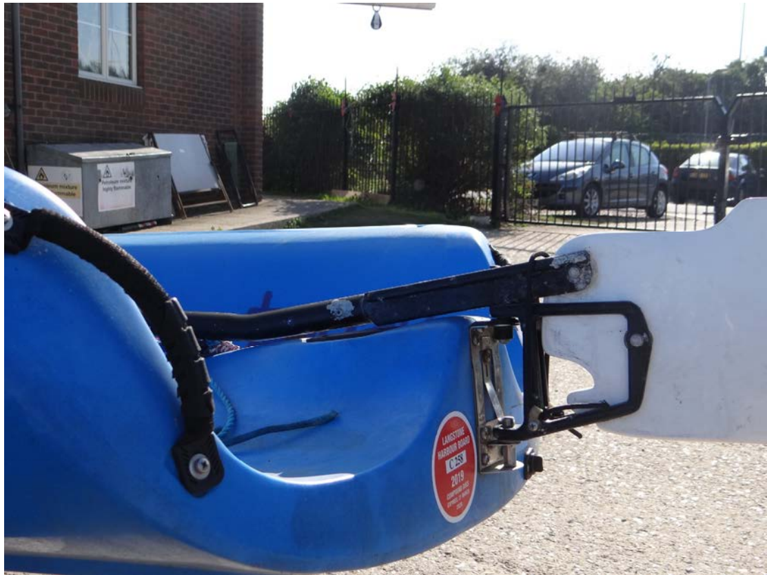
Pic 7 Rudder attachment
