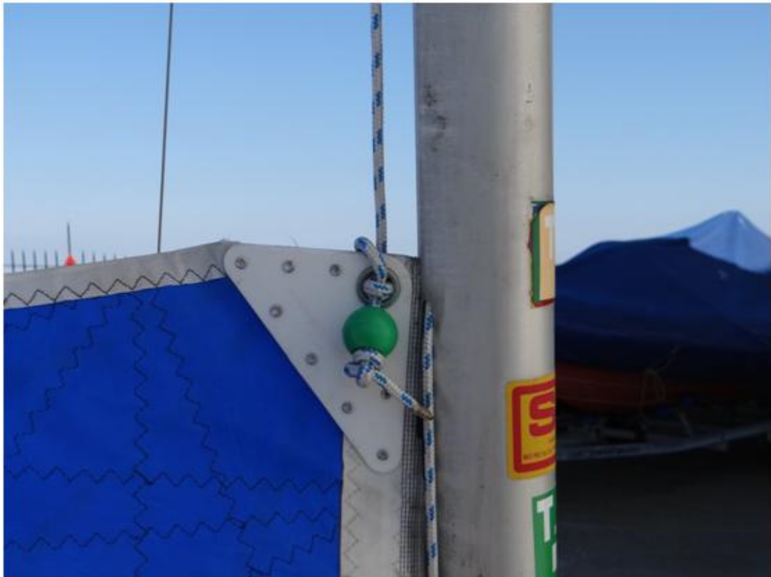
Pic 6 – Attaching main halyard
